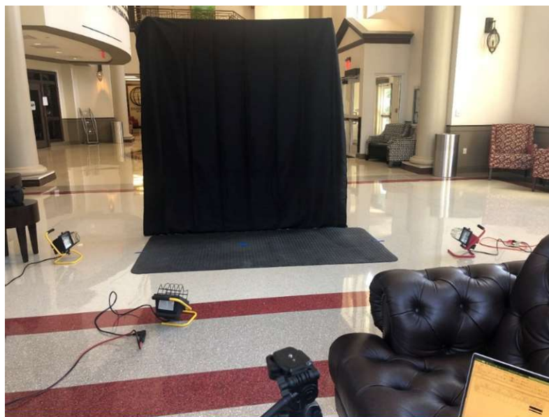
Figure 11: Experimental testing set-up for high-speed camera and four lights
