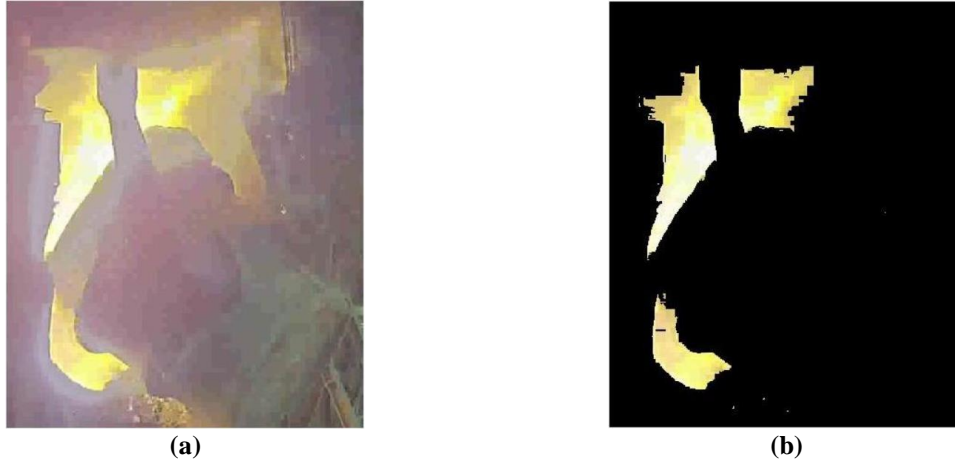
Figure 4. Example of flame segmentation: (a) original image and (b) after flame segmentation is applied.
