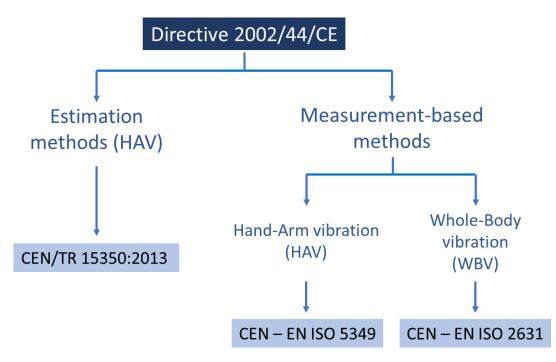
**Figure 2.** Schematic view of the applicable technical regulations for hand-arm transmitted vibration (HAV) and whole-body vibration (WBV).
