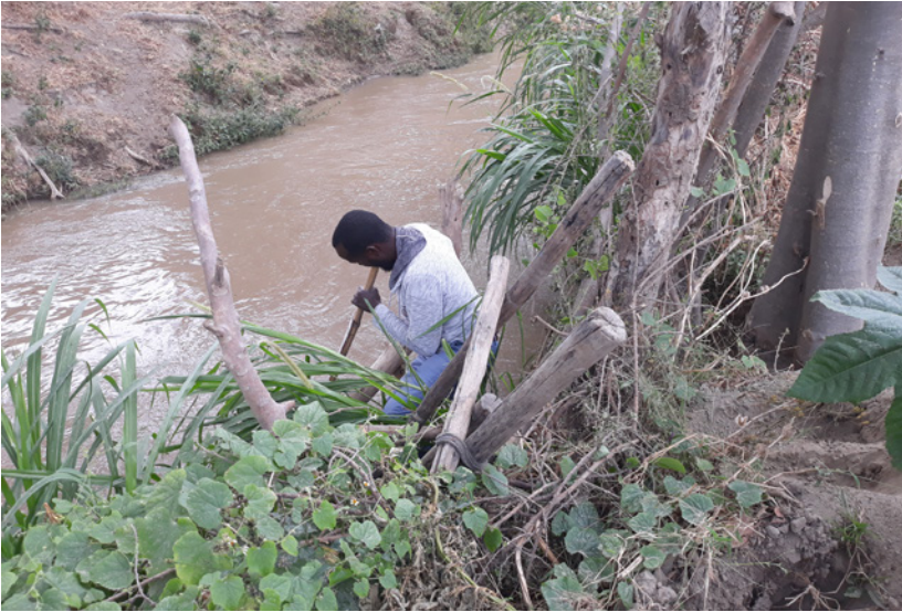
Figure 11. Observers taking measurements at gauging stations. (a) the observer at Desta Abijata (Station number 5) must climb a ladder to measure the water level with a stick, and (b) the observer at Meki at Meki Village (Station number 1) deals with a dirty and dangerous measurement location.
