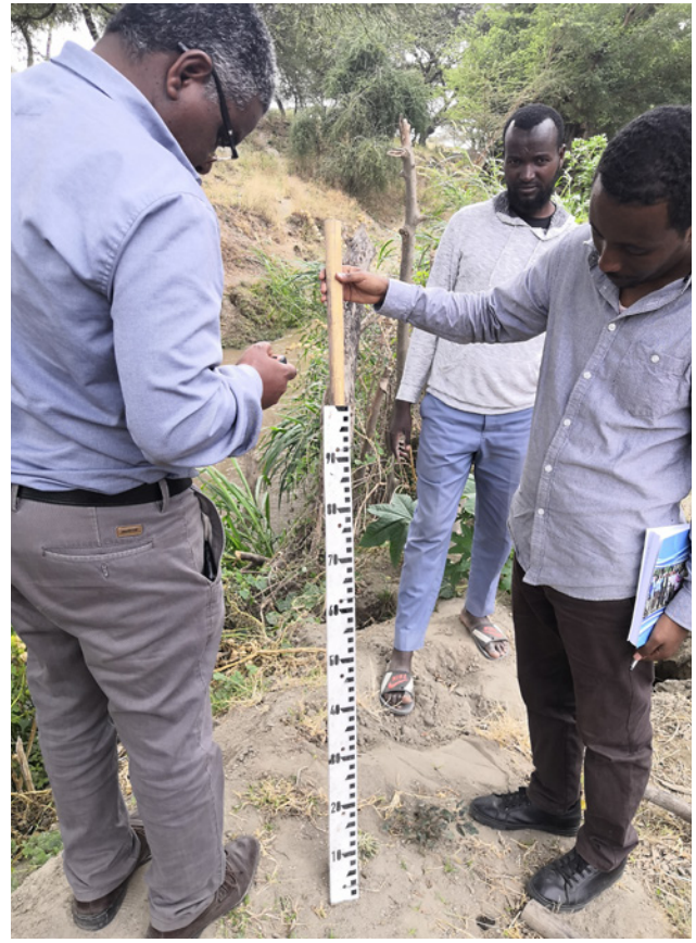
Figure A5.3. The observer uses a stick to measure the water level at Desta Abijata gauging station.
