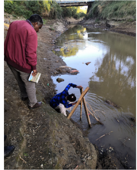
Figure 11. Observers taking measurements at gauging stations. (a) the observer at Desta Abijata (Station number 5) must climb a ladder to measure the water level with a stick, and (b) the observer at Meki at Meki Village (Station number 1) deals with a dirty and dangerous measurement location.
