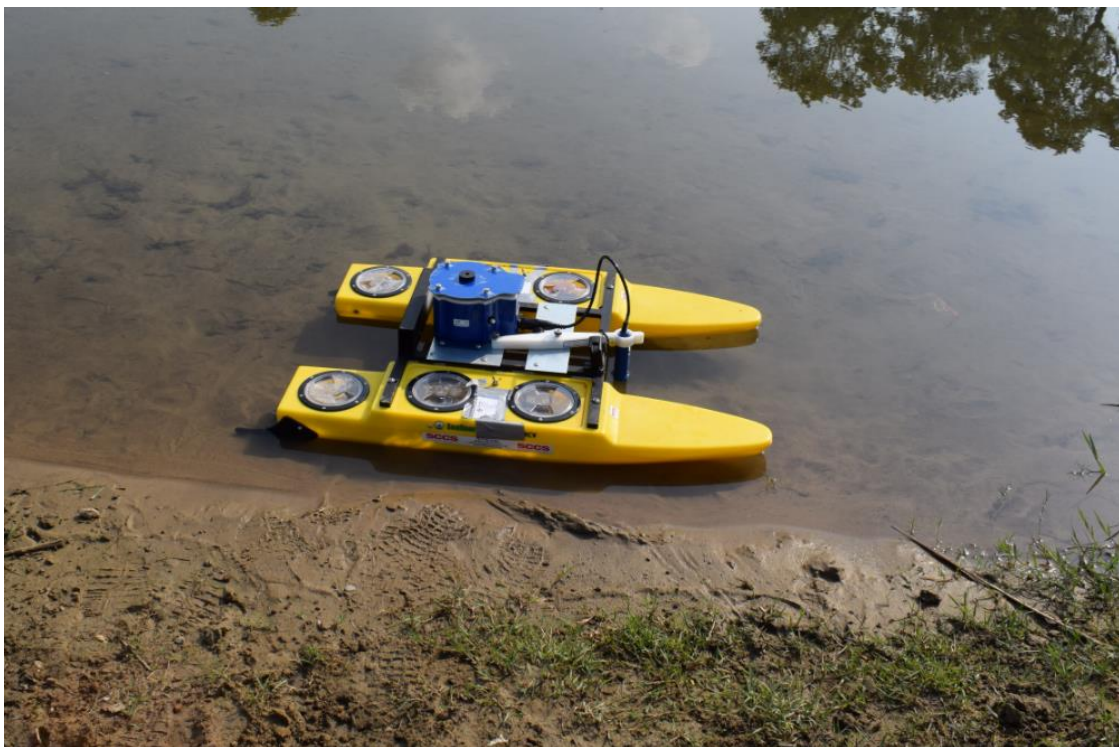
Figure 3.13: The Seafloor HyDrone RCV with attached ADCP for gauging wider and deeper channels (taken on 16/05/2018).
