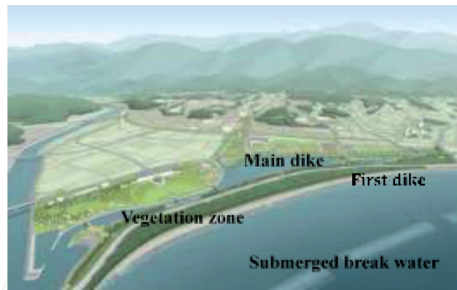
Figure 5. New protection system along the coast of the city (source: the city office).
