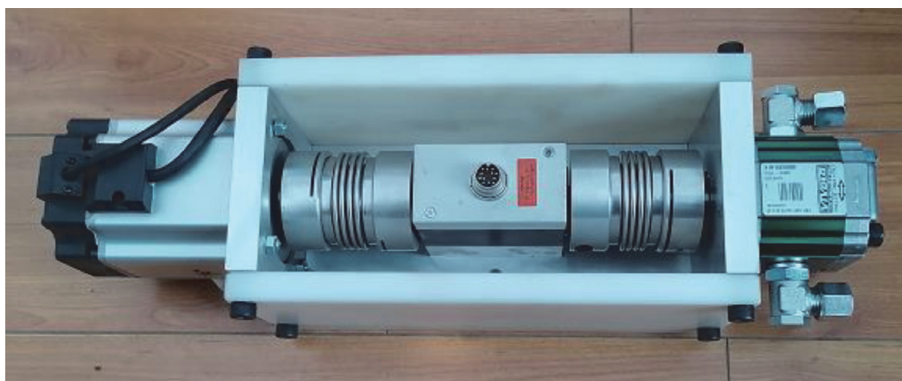
Figure 43. Servopump for hybrid servomechanisms designed in the Fluid Power Systems Laboratory of U.P.B. [30].
