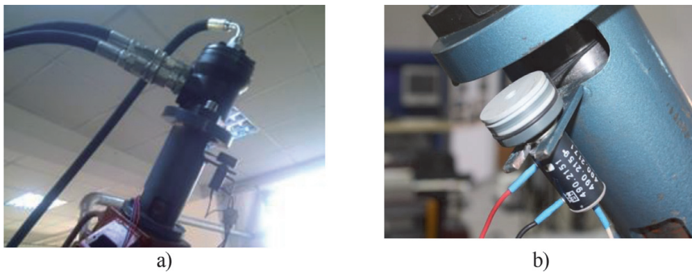
Figure 28. Hybrid steering servo system driven by an ORBIT motor in close loop: (a) driving system view; (b) rotary feedback potentiometer driven by the motor.
