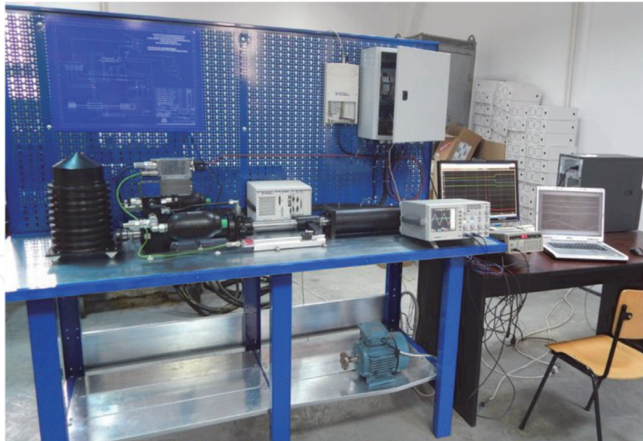
Figure 22. Test platform for identifying the digital servovalve performance [17].
