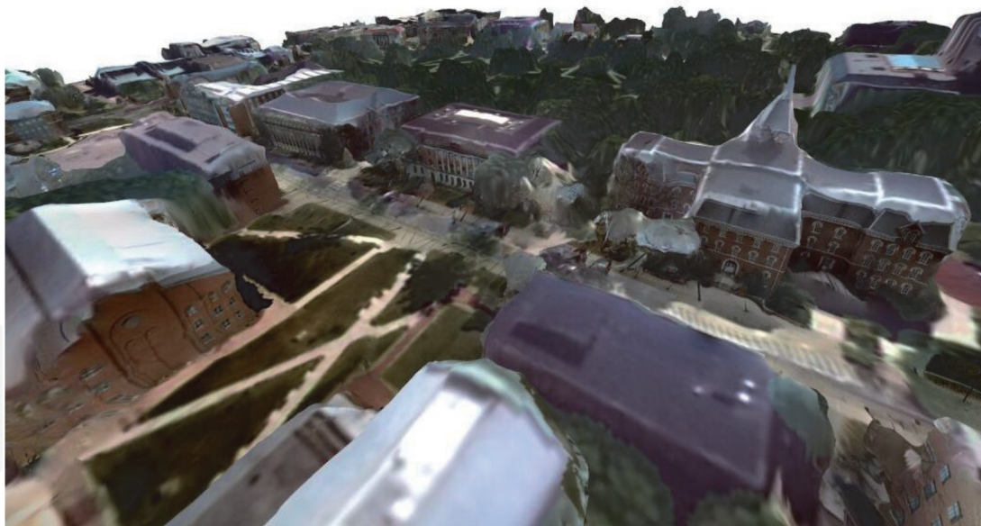
Figure 15. A screenshot of the generated textured mesh of the OSU campus area using our proposed pipeline, which includes information from the top-view and details on the facades.
