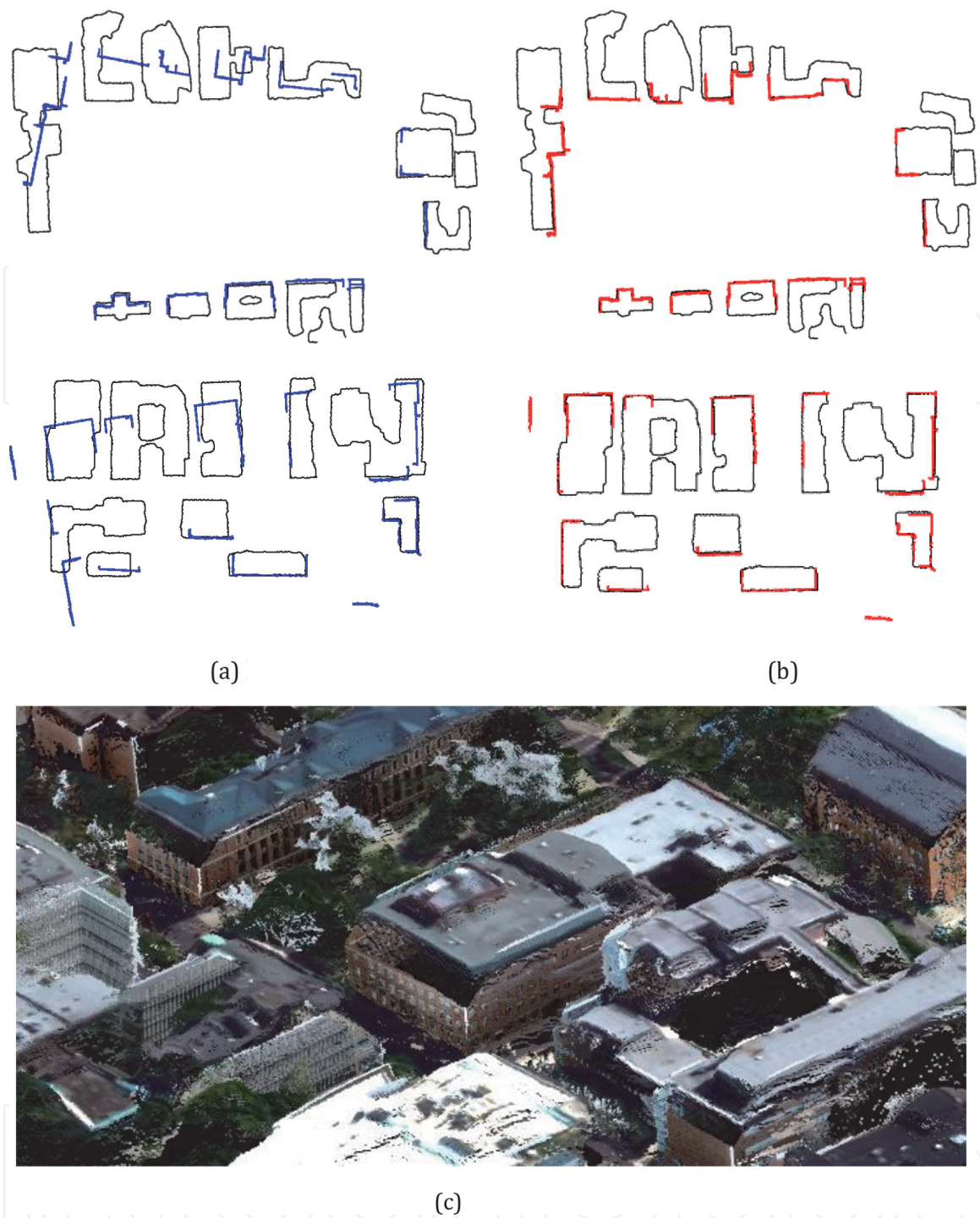
Figure 13. Registration result of ICP (a) and our method (b) on the distorted ground-view trajectory. (c) Part of the registered ground-view point clouds generated on 150 k Go-Pro images.
