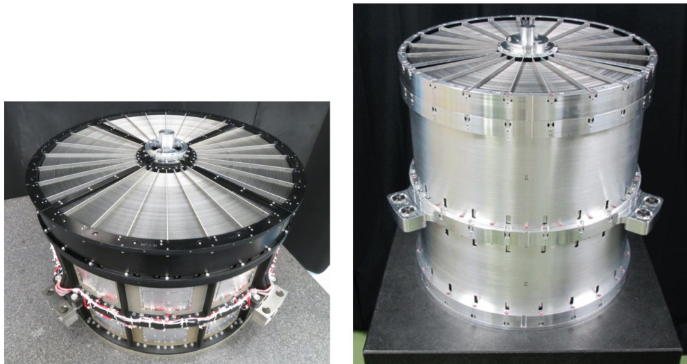
Figure 4. Photographs of flight models of (left) Soft X-ray telescope, SXT-S and (right) hard X-ray telescope, HXT-1.
