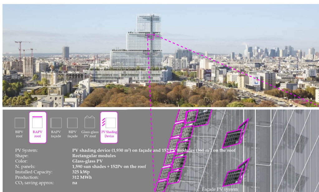
Figure 9. Paris Courthouse east façade (photography with permission of author Sergio Grazia) (on the top); Integration and characteristic of PV systems (on the bottom).
