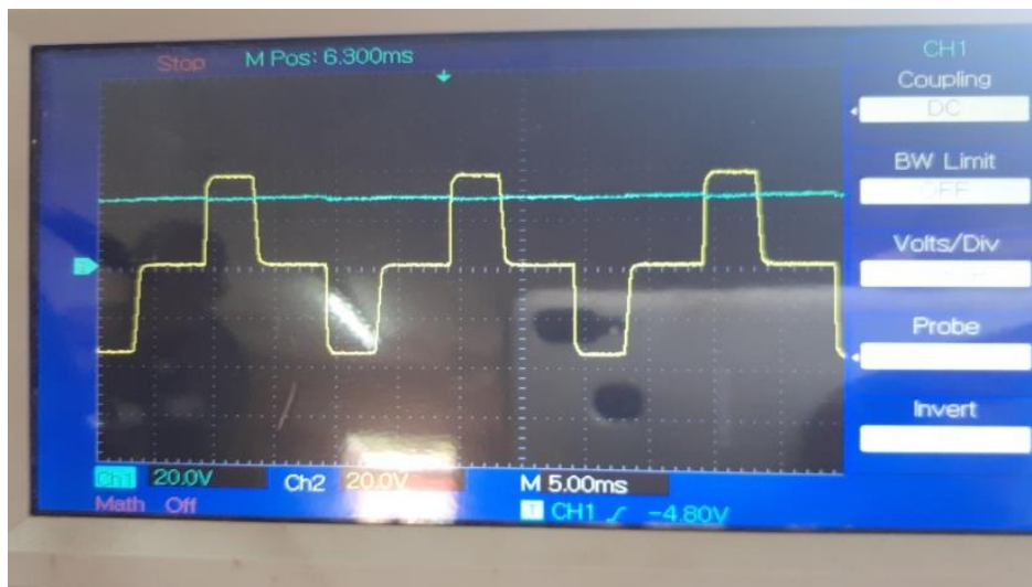
Fig. 4 Output waveform of the inverter on no load
