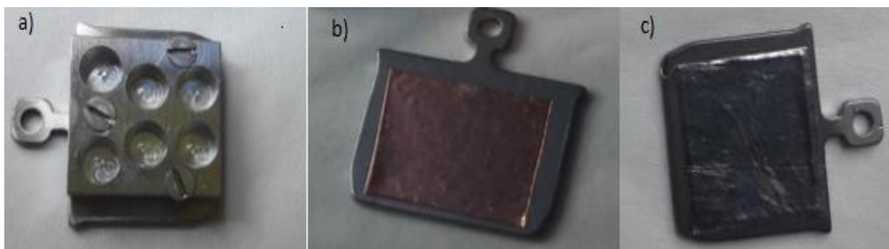
Figure 3.4: Three different types of sample holders for XAS experiment. The first picture with indium tape on the top of the stainless-steel sample holder and the stainless-steel pallet over it (a). The second picture with copper tape on the top of the stainless-steel sample holder (b). The third picture with indium tape on the top of the stainless-steel sample holder (c).
