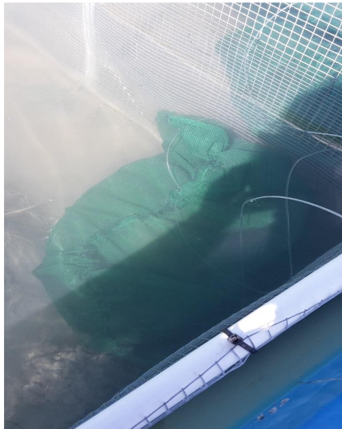
Figure 2.2. Photograph of one shade-cloth bag sewn together using fishing wire. The bags were tied onto a mesh cage.
