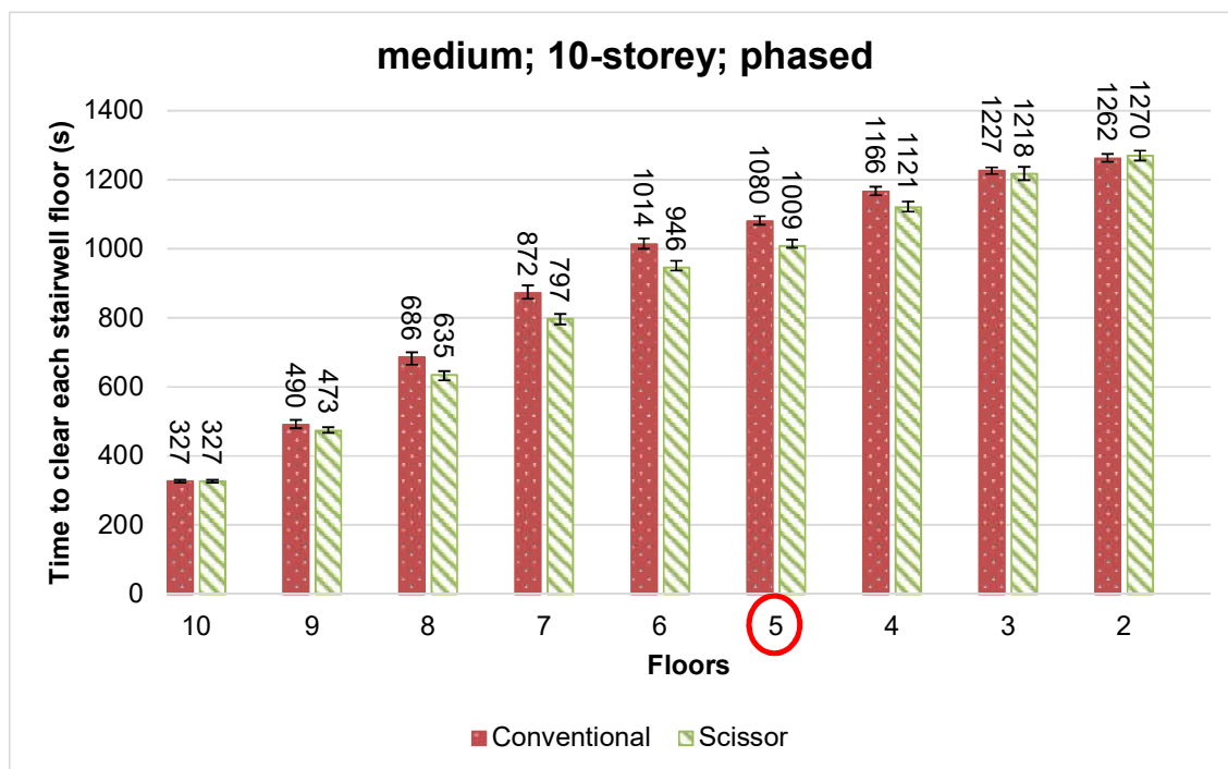
Figure 5-21: Time to clear floors of conventional and scissor stairs (medium; 10-storey; phased)
