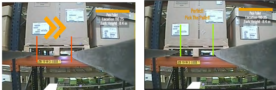
Figure 4.4: Fork horizontal alignment
