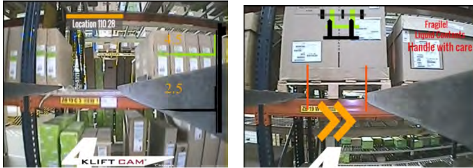
Figure 4.6: Fork horizontal alignment
