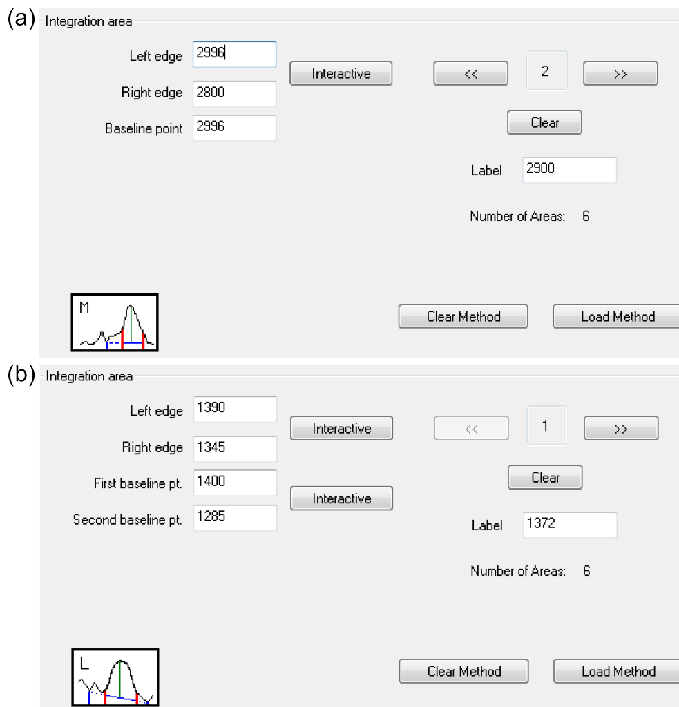
Figure 100: Settings for integration routine of I_{2900} and I_{1372} to determine TCI in OPUS 7.2.
