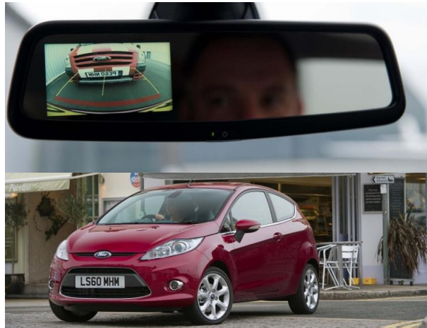
Figure 2.1.1: Parking assist using AR Technology on the Ford Fiesta Credits: Ford Fiesta 2011 Brochure [6]
