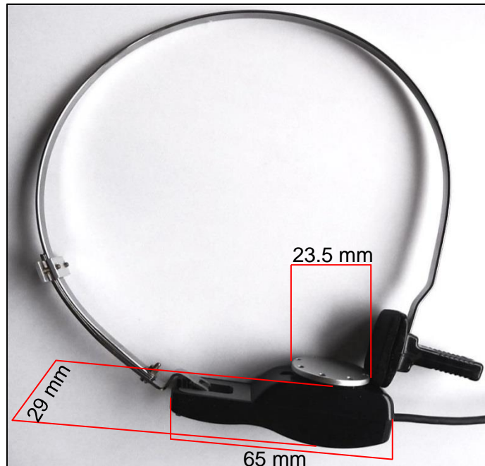
Figure 38. Final transducer and headband set-up showing dimensions of the transducer.
