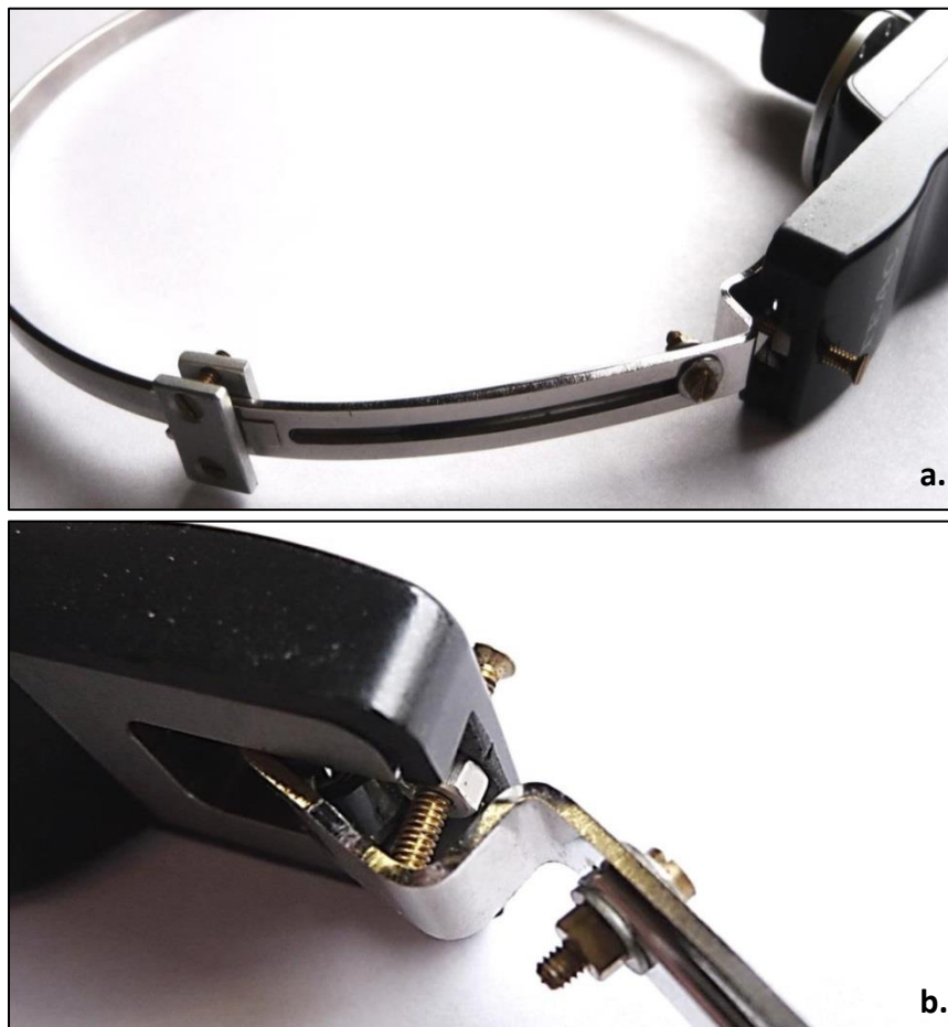
Figure 37. a). The attachment of the P-3333 headband to the TEAC transducer using the bracket of the TEAC transducer, two small metal plates joined by two screws and a third screw at the distal end of the headband. b). shows a close-up view of the screw inserted through the top of the transducer casing to consistently hold the transducer at the correct angle against the head.
