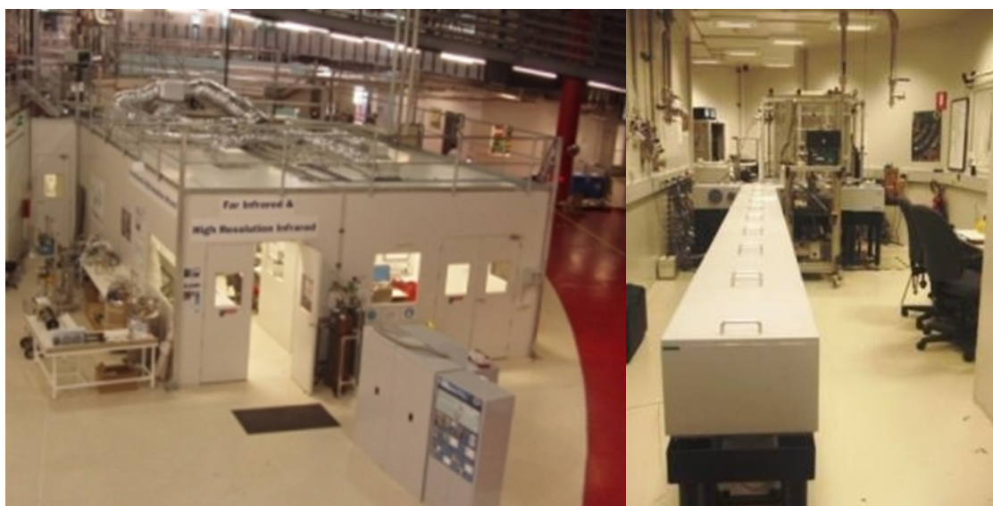
Figure 18; The Far-IR beamline at the Australian Synchrotron, and the Brüker IFS 125/HR FT spectrometer
