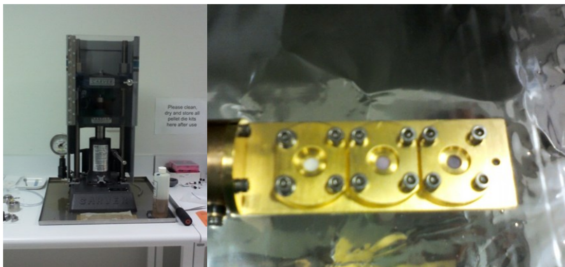
Figure 19; Samples were prepared with a pellet press and subsequently loaded on to the \text{LN}_2 cryostat sample holder
