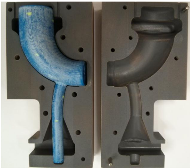
Fig. 2 Test mould with the internal mould (blue) placed in the external mould (grey)
