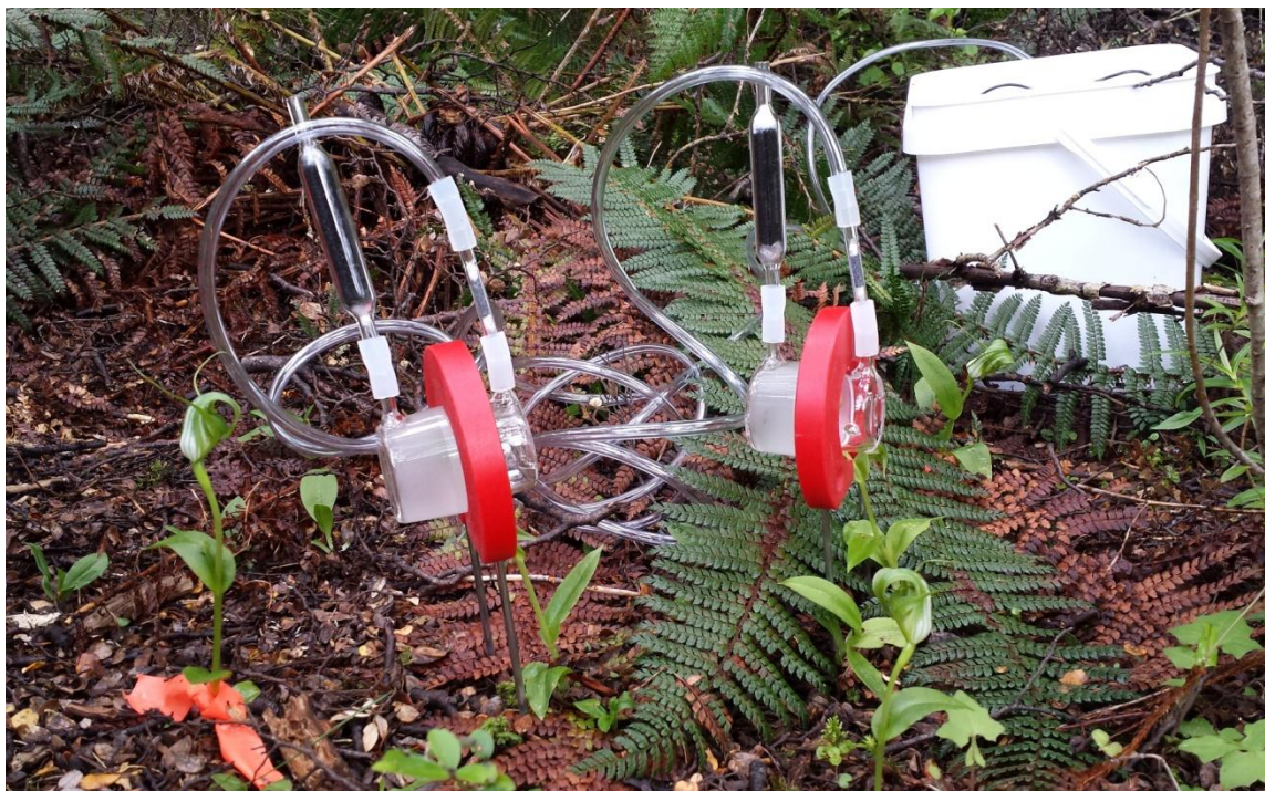
Figure 4.2 Headspace volatile collections of P. oliveri flowers at Greyney's Shelter. In the picture, the glass chambers are set up over the flowers. The charcoal tube (larger tube), and the Tenax trap (small tube) which is connected to the floral chambers and the battery powered vacuum pump (within the white plastic container) via silicon tubing. Picture taken by Liezl Thalwitzer.
