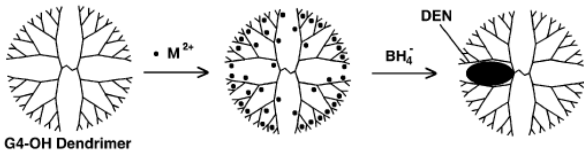
Figure 2.8 A scheme of formation metal nanoparticles inside a dendrimer. Adapted from Chemistry of Materials 26(1), 72-83. Copyright American Chemical Society.
