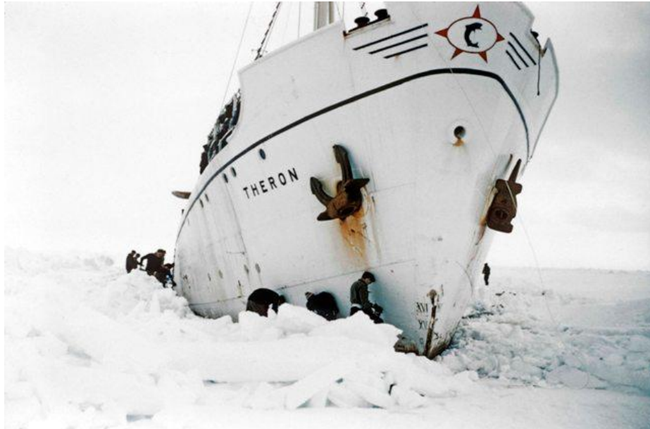
Figure 19: Theron beset in the Weddell Sea pack-ice – January 1956 The men shown are working with picks, poles and shovels to try and free the ship. Photo: George Lowe
