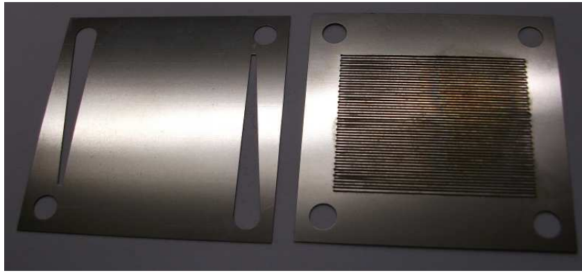
Fig. 1: Feed shim on left, microchannel shim on right
