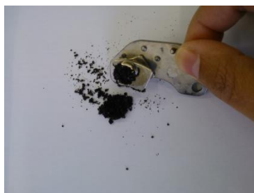
Figure 6.17-Response towards a Nd 2 Fe 14 B magnet of crystals of [C 3 (NEt 2 ) 3 ]FeCl 4 .
