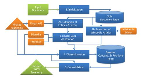
Figure 17: System View of F-STEP
