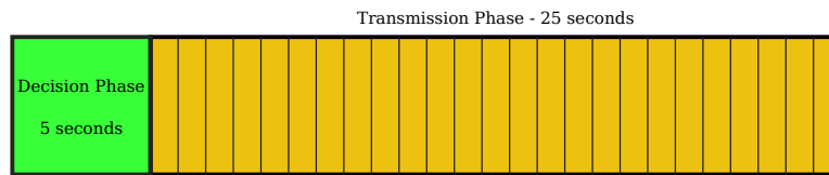
Figure 3.2: Round model, split into the Decision and Transmission phases
