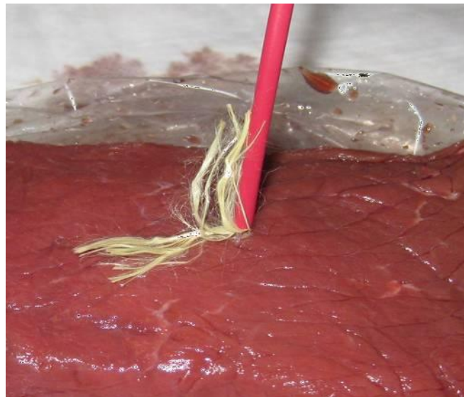
Figure 5.3: Multi-mode fibre undergoing laser heating
