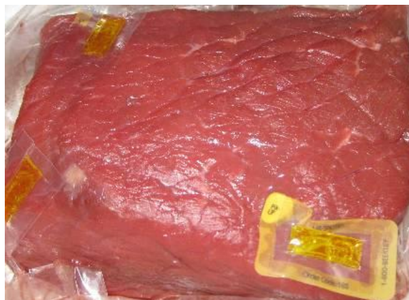
Figure 5.5: Co-ordinate tabs fixed to new bovine phantom
