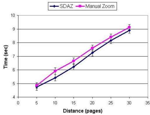
(a) Mean target acquisition times against distance for SDAZ and rate-based scrolling with manual zooming in the text interface.
