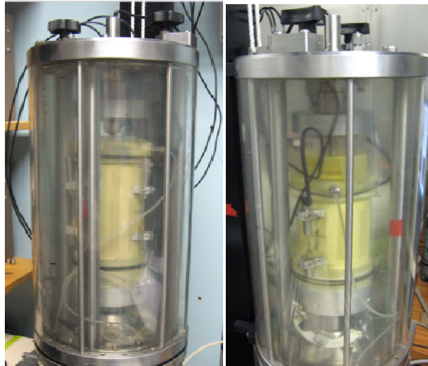
Figure 4-7: Sample in triaxial apparatus- knob-and-dimple top cap (left), top cap with vylastic sleeve (right).
