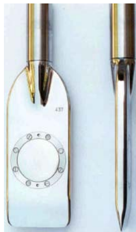
Figure 2-13: Flat plate dilatometer (Marchetti et al., 2001).
