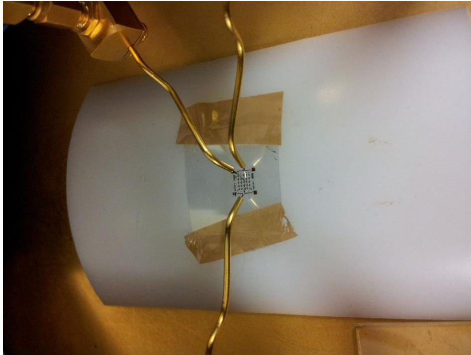
Figure 7.6 – Testing setup for the mechanical bending of substrates at a radius of 30 mm.
