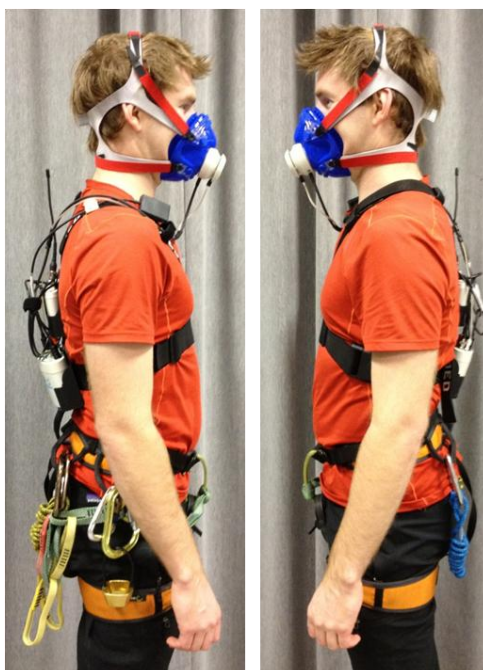
Figure 3.10 Cosmed K4b 2 harness configuration lateral views.
