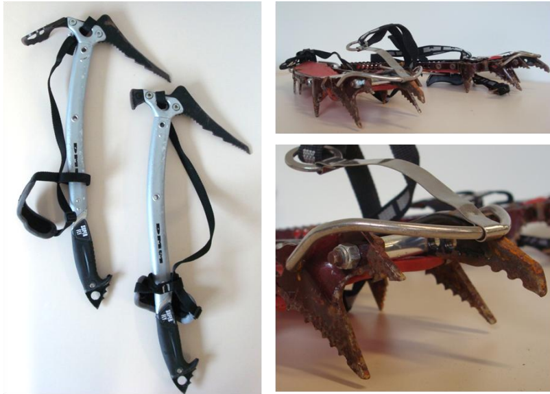
Figure 2.14 Specialized ice climbing equipment; climbing axes (left) and rigid crampons featuring front points (right).
