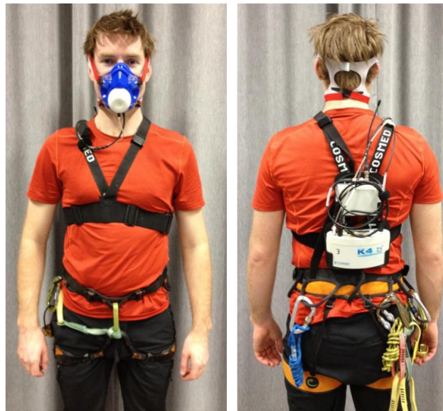
Figure 3.9 Cosmed K4b 2 harness configuration anterior and posterior views.
