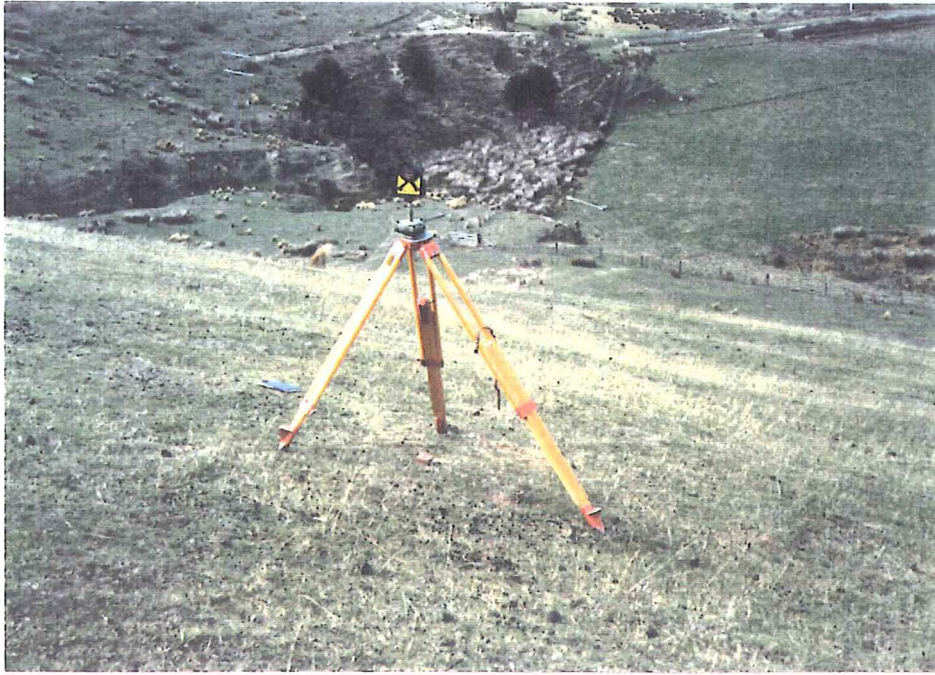
Figure A1.3 Tripod mounted prism used for displacement surveying.
