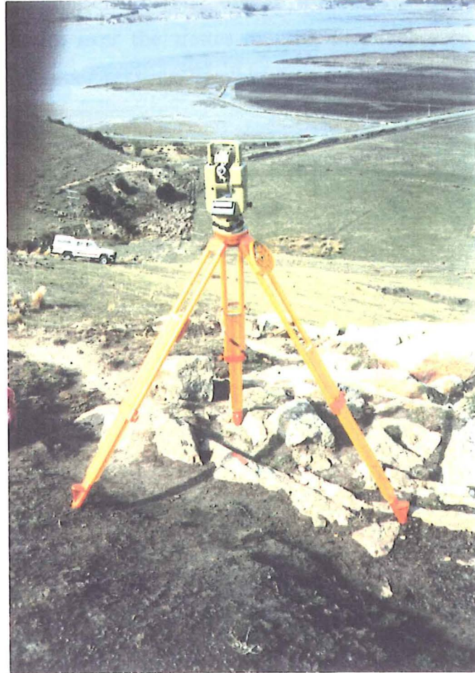
Figure 3.25 Survey Control Station (S1)- position fixed permanently by pop-verting webbing to bedrock surface.
