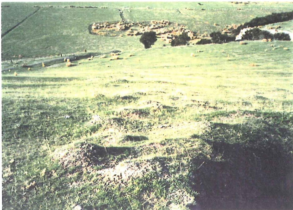
Figure 3.6 Slope Deposit Trailing from Flanks of Failed Ground- photograph taken from the downslope portion of the eastern flank of the investigated failed ground complex.
