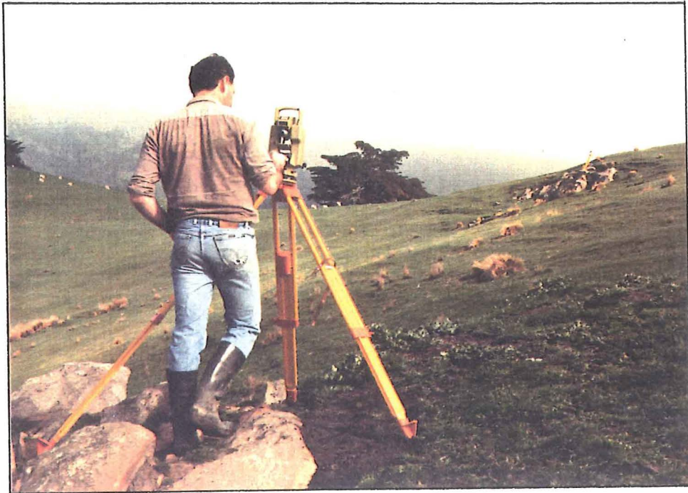
Figure A1.1 Tripod mounted EDM, used for all surveying. Base line (S1-S2) runs between the two rock outcrops.
