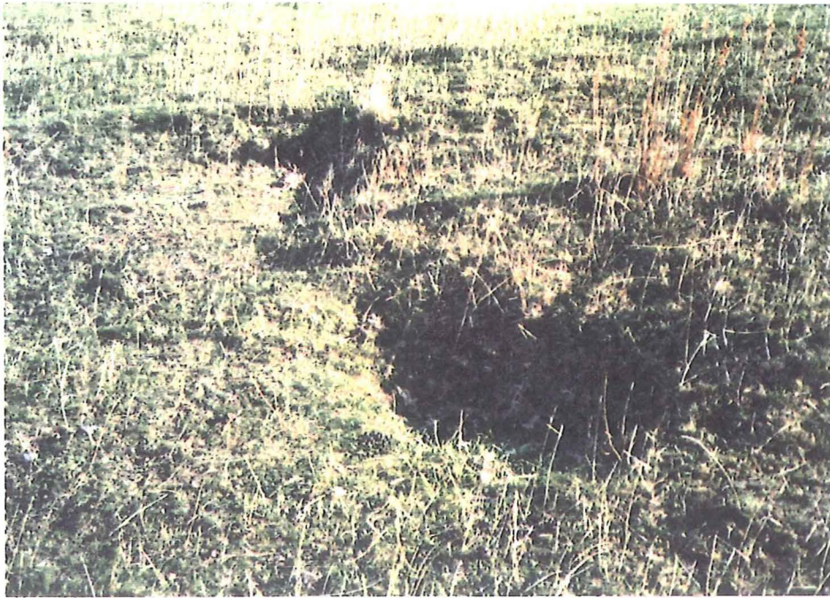
Figure 3.11 Slump Block with Associated Head Scarp- upper eastern part of investigated failed ground. Note: Pit 1 was dug across this slump feature.
