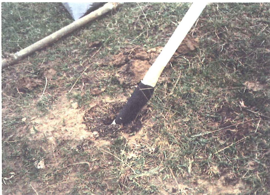
Figure A2.2 Slotted end of piezometer wrapped in geotextile
