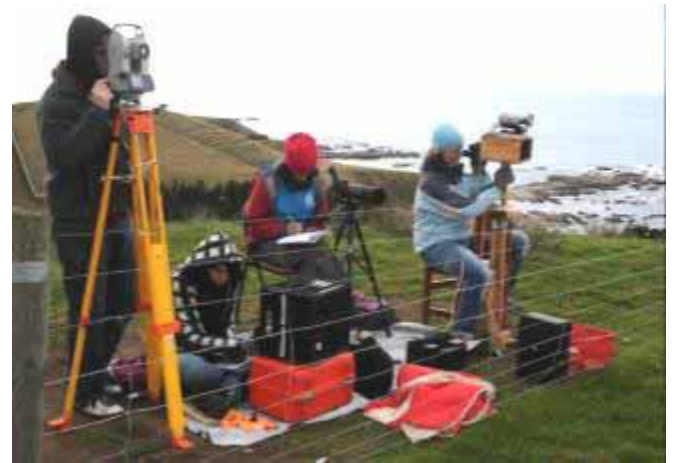
Figure 2.2. The research team tracks whales from the shore station. From left to right: theodolite operator, data logger (laptop), note taker and digital video binocular system operator.
