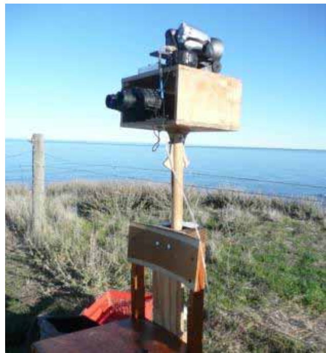
Figure 2.4. Video system. Digital video binocular system is used to monitor and track whales and vessels.
