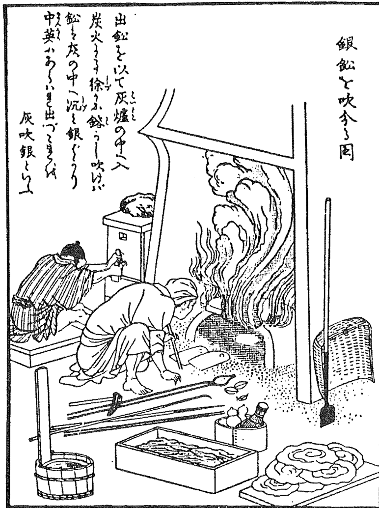
The cupellation process as practised in Japan. From Masuda Tsuna, Kodō Zuroku (1801); reproduced in Needham and Lu, Spagyrical Discovery and Invention: Magistrates of Gold and Immortality , p. 37.
