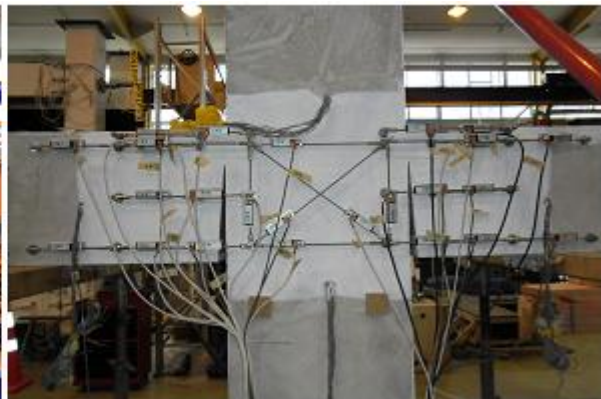
(j) Linear potentiometer installation
