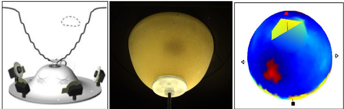
Figure 1.1: Key steps of the DIET Imaging procedure: (1) Excite the breast at low frequencies [left], (2) Image surface motion with digital cameras [middle] and (3) Calculate motion disturbance for diagnostic analysis [right]. Embedded in this breast phantom is 20 mm stiffer inclusion at 6-7 o'clock which can be easily identified
