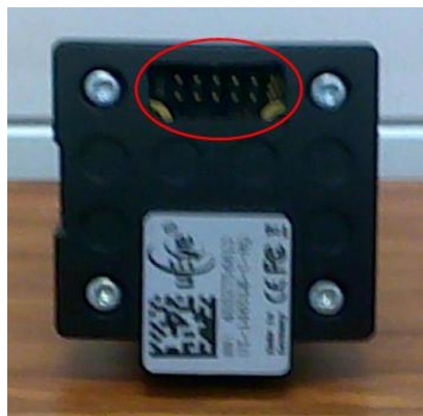
Figure 2.3: Showing the pin configuration extended as a result of hardware modification in the test camera providing a control signal for exposure. The objective was to convert rolling shutter into global start rolling shutter
