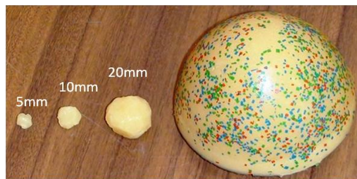
Figure 10.1: Silicone breast phantom with examples of stiffer inclusions embedded inside
