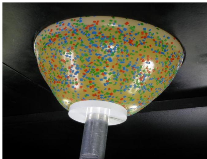
Figure 3.2: Stage-1 DIET prototype image showing specular reflections from the highly reflective surface of the silicone breast phantom during in vitro trials
