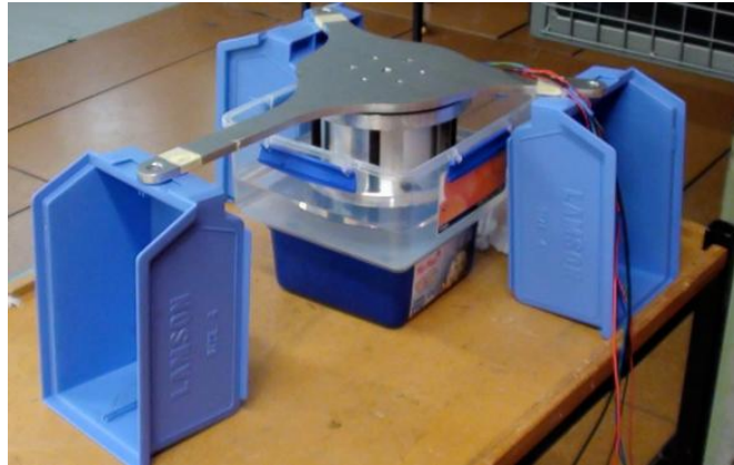
Figure 4.11: Showing experimental set up for testing silicone padding as vibration isolation solution
