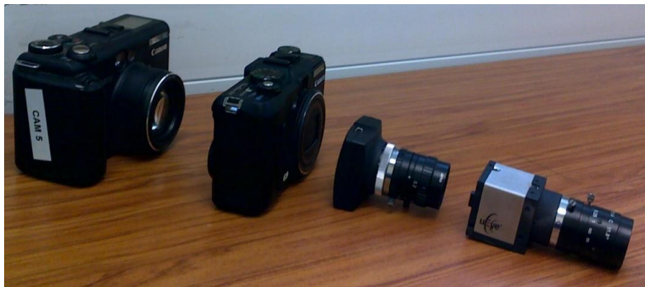
Figure 2.4: Evolution process of digital cameras for DIET, starting from left Canon G5, Canon G9, IDS UI 1465 LE-C, IDS UI-2250 SE-C with C mount lens
