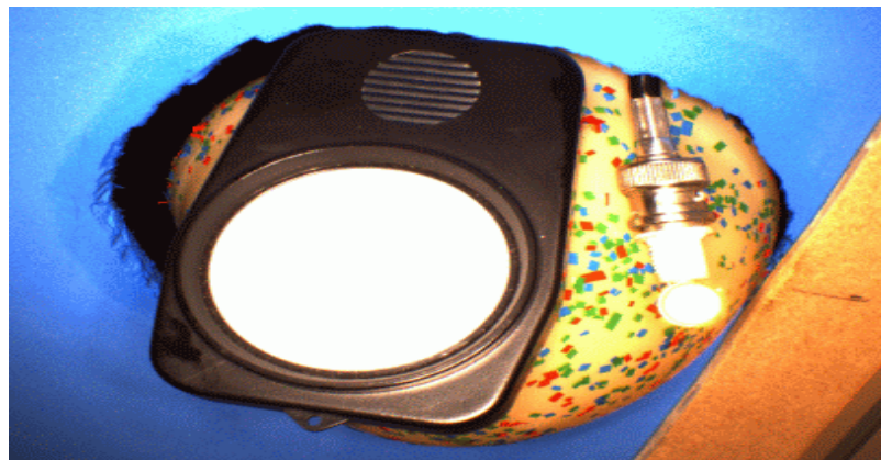
Figure 3.9: Showing calibration test settings with a photodiode and luxmeter applied in the darkroom environment. LED strobe system is in operation
