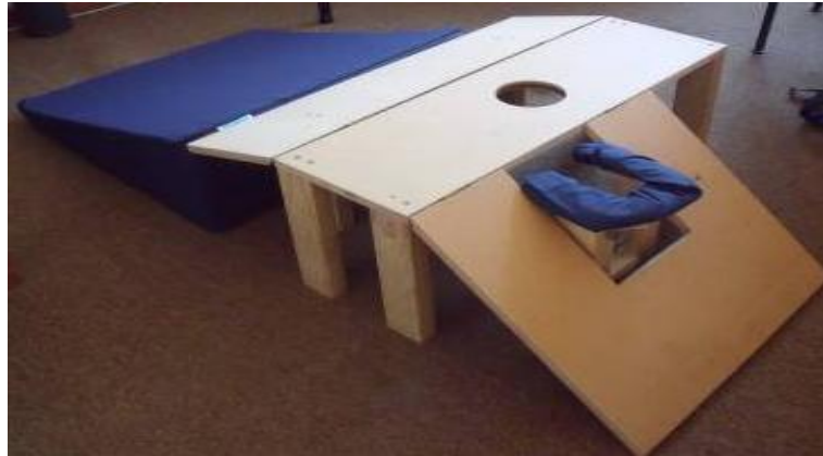
Figure 6.6: Wooden mock up device constructed to evaluate general space requirements and functionality
