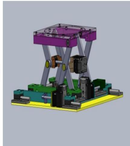
Figure 5.2: Solidworks representation of lift table concept; fully retracted (left) and fully extended (right)
