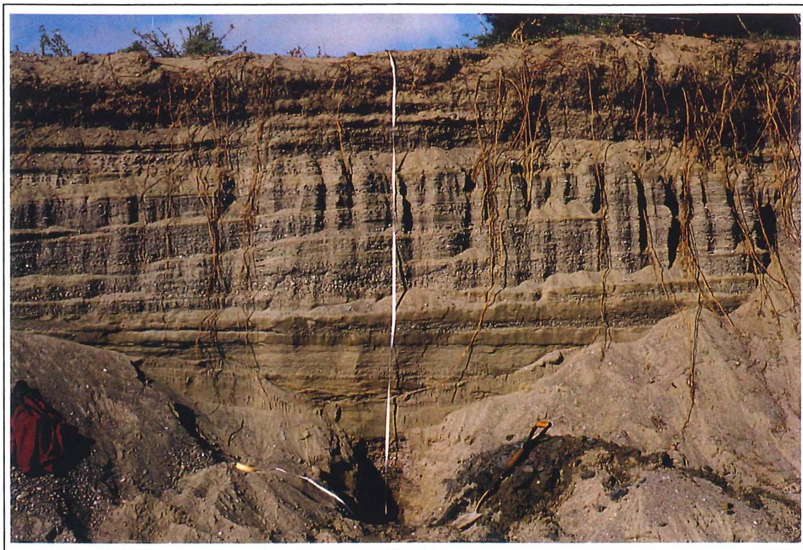
Figure 3-6. Photo of Taumutu Gravel Pit south wall showing eastward dipping sandy gravel layers which downlap a series of horizontal beds of sand and gravel. Note the blue silty clay which occurs at bottom of the hole. The elevation at the top of the face is c. 6.5 m. Note spade for scale. Taken looking southeast at M37 588 065.
