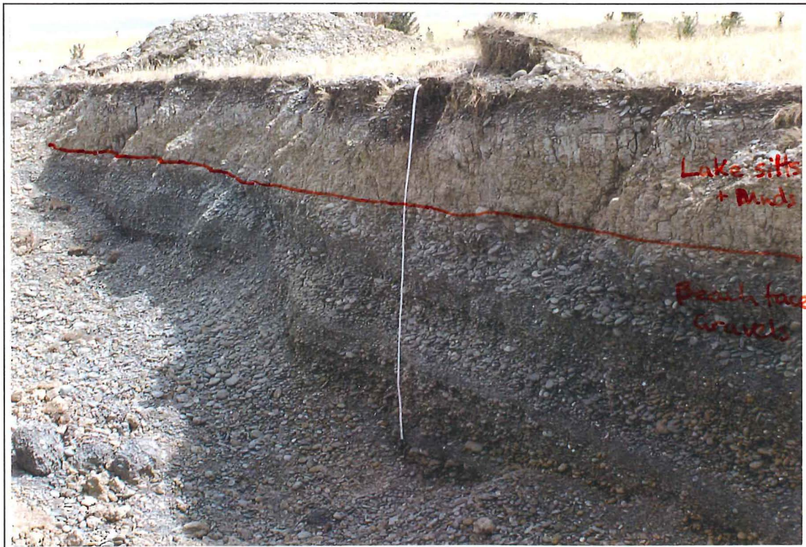
Figure 3-4. South facing wall of large pit at M36 768 102. Note the muddy gravel overlying a silty clay layer, which appears to be sitting on a truncation surface developed on well bedded gravels. The height of the face is 1.6 m.
