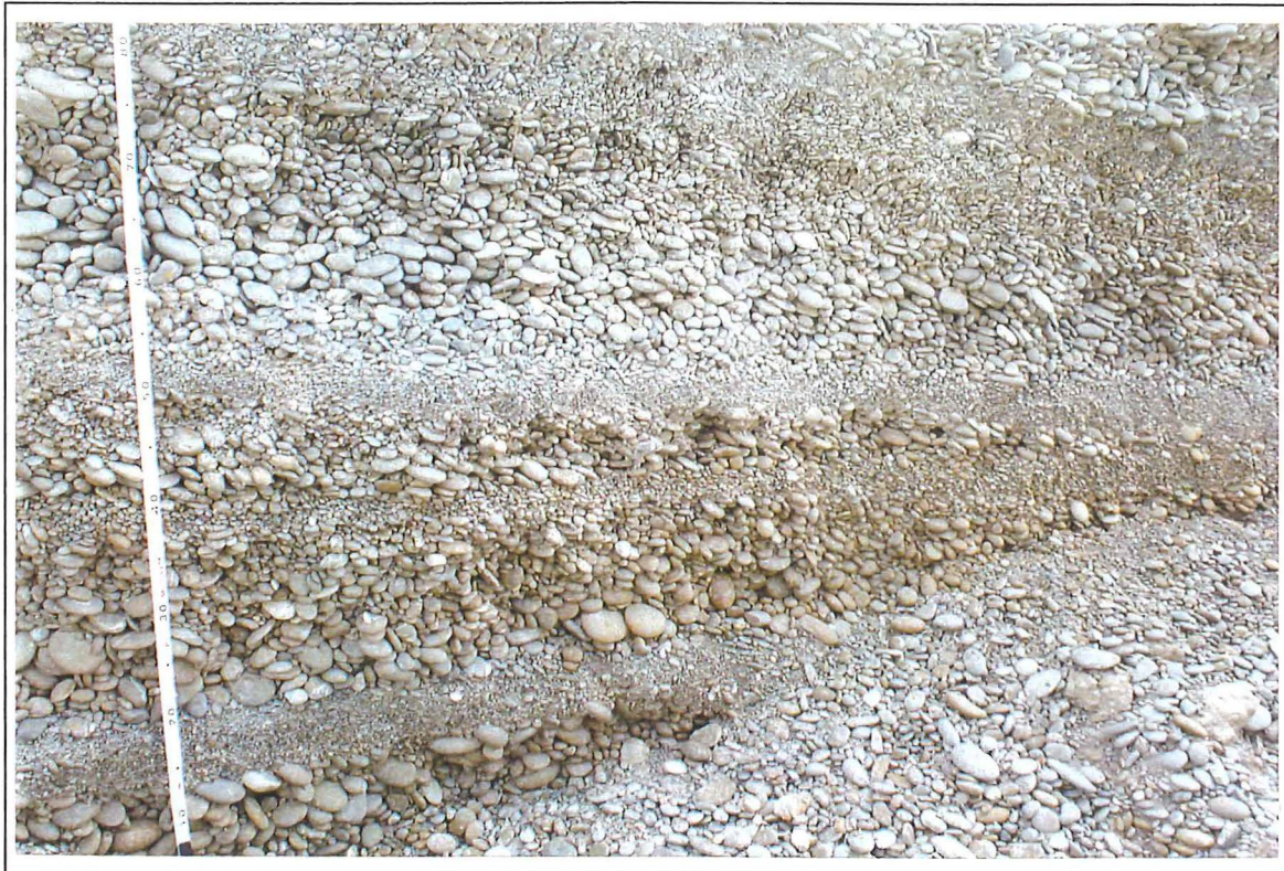
Figure 3-5. Photograph of a section of the truncation developed in the well bedded gravels in the pit at M36 768 102. The truncation and overlying beds have an apparent dip of 4^\circ east, the gravel beds below the truncation have an apparent horizontal attitude. All the beds are actually dipping to the south at 4-7^\circ . Photograph height is 0.8 m.
