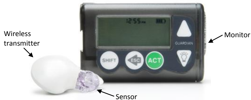
Figure 2.1 The Medtronic Guardian Real-Time CGM - a commonly available and widely used CGM device.
