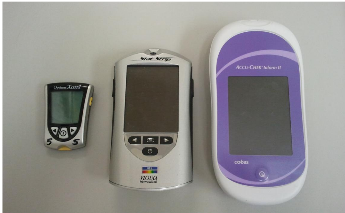
Figure 11.2 The three glucose meters used in this study. From left to right: Abbott Optimum Xceed, Nova Statstrip Glu, Roche Accu-chek Inform II.
