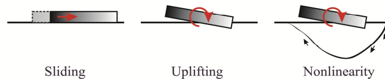
Figure 10-1. Possible types of soil-foundation interface nonlinearity.
