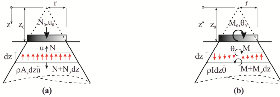
Figure 5-4. Truncated semi-infinite cone with static and dynamic equilibrium of infinitesimal element: (a) translational cone with nomenclature for vertical motion and, (b) rotational cone with nomenclature for rocking motion [2].
