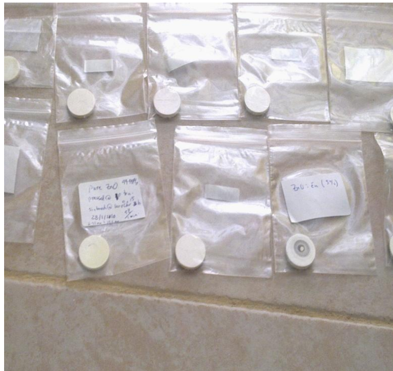
Figure 2.6 One-inch diameter PLD targets of ZnO doped with Er and Eu atoms.
