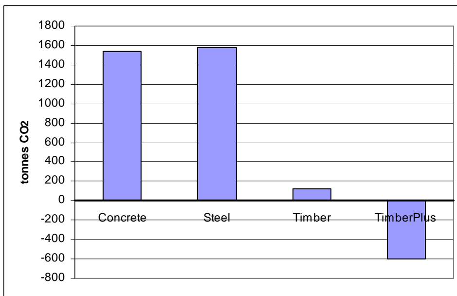
Figure 9.4. Net GWP emissions for the materials in the four buildings, assuming permanent storage of carbon in wood products. Data from LCA analysis in Chapter 6.
