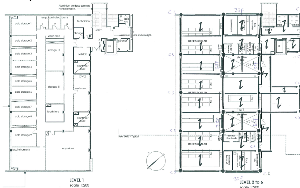
Figure 4.7: Sketches of the layout of Steel building structure (right) compared with the layout of the actual laboratory concrete structure (left).
