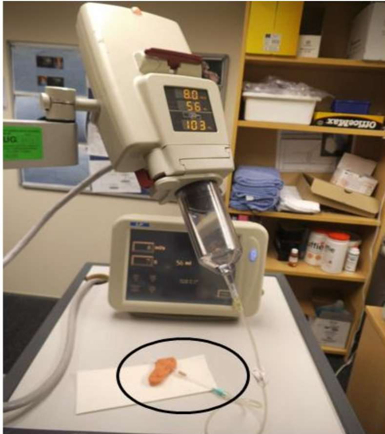
Figure 4-6: Digital injection system that was used to inject water during reflexive swallowing task. The circled item is the tube through customised dental bite-block to facilitate water injection in the pharynx during reflexive swallowing.
