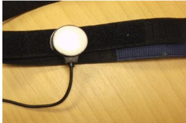
Figure 4-8: The pulse transducer consists of piezoelectric element which was attached to a strap to position the transducer during the swallowing tasks.
