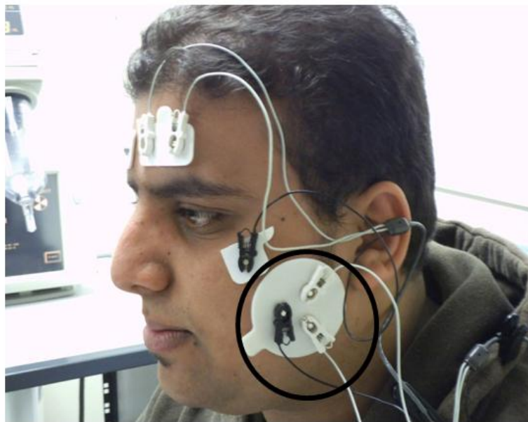
Figure 4-12: Electrodes placement for the jaw movement task.
