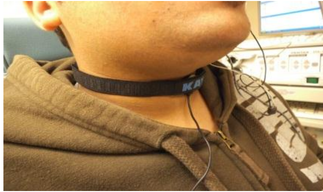
Figure 4-16: The piezoelectric transducer and its placement over the thyroid cartilage to trigger TMS.
