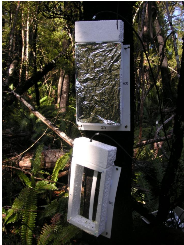
Figure 3.1: Setup of enclosures on one of the sampled trees (before netting was added). Wires are attached to temperature probes at the top of each enclosure and run down to the datalogger at the bottom right of the photo.
