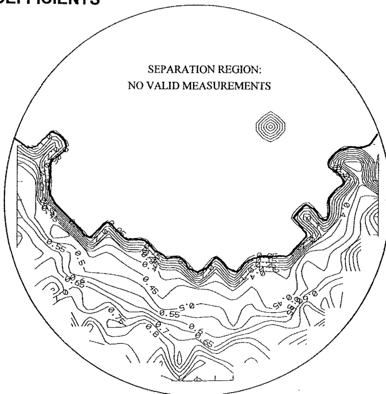
FIGURE 5.16 IMPELLER FLOW CONDITIONS: IVR \approx 0.32 : Re = 195\ 000
