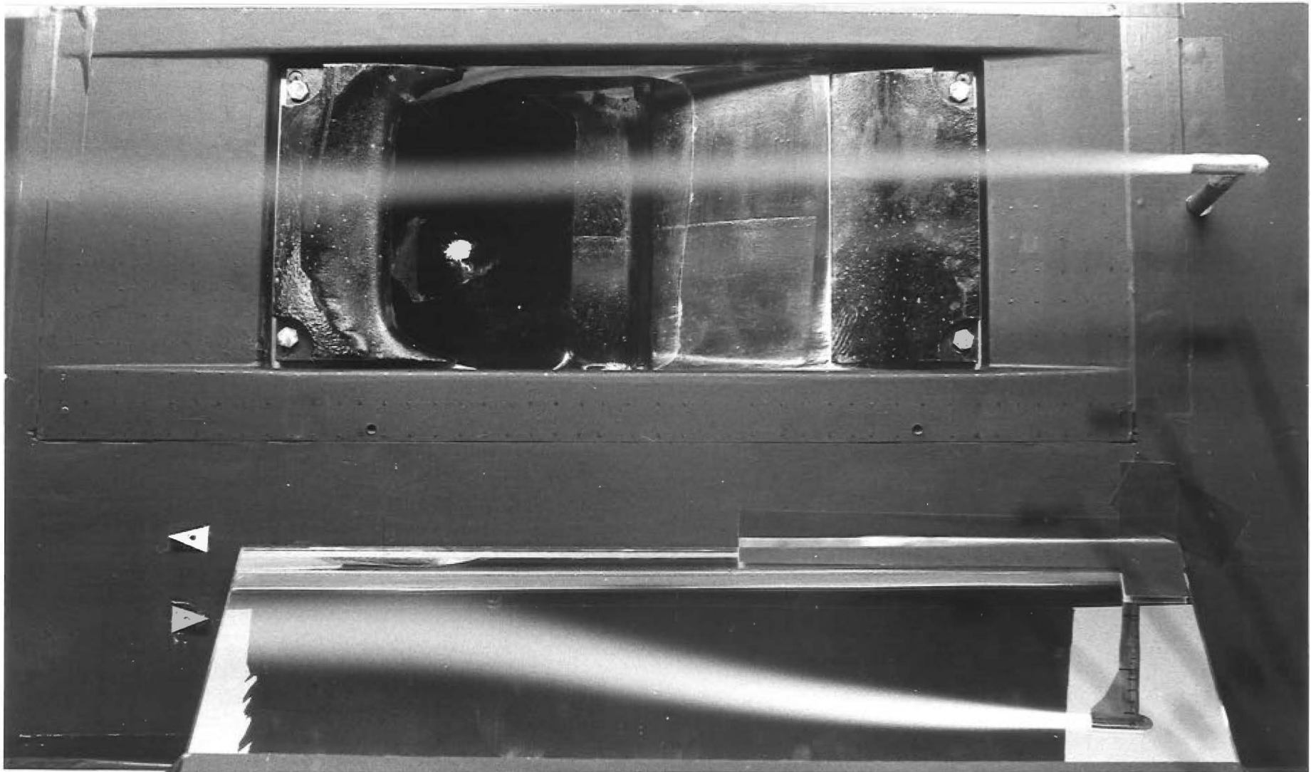
FIGURE 4.2 EXAMPLE OF THE SMOKE PLUME STREAMLINE INVESTIGATING THE STREAMTUBE
