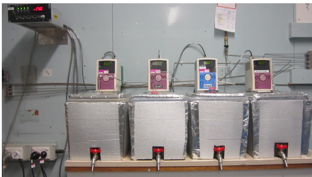
Figure 3.9: Four water baths containing submerged diffusion system controlled by temperature controllers.
