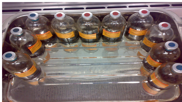
Figure 5.1: Batch mode, serum bottle experimental set-up (inside a 30 °C incubator).
