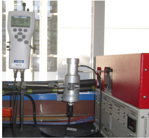
Figure 3.15: Carbon dioxide probe connected online with the outlet of GC and read out records the measured carbon dioxide.
