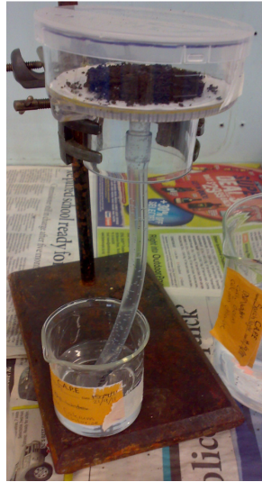
Figure 3.3: Photo of Zap Cap filter used to determine the water retention curve
