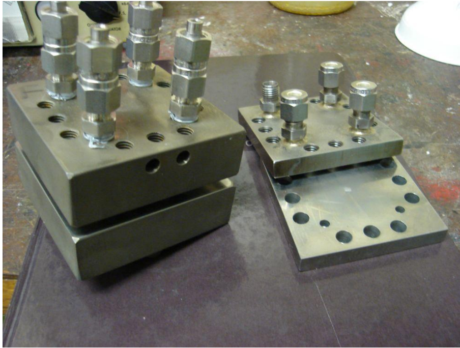
Figure 37: Second reactor model constructed from Stavax on left, in comparison to stainless steel model on right
