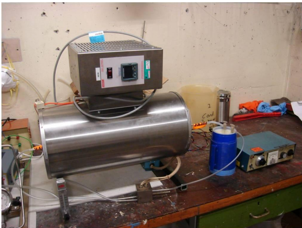
Figure 46: Physical arrangement of TPR system
