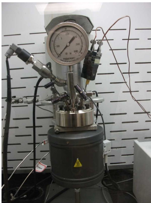
Figure 2: Reactor installed in rig showing electrical and plumbing connections and heating element in place
