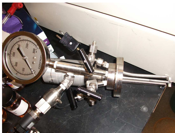
Figure 4: Inside view of the reactor showing the gas inlet, the thermocouple well and the stirrer
