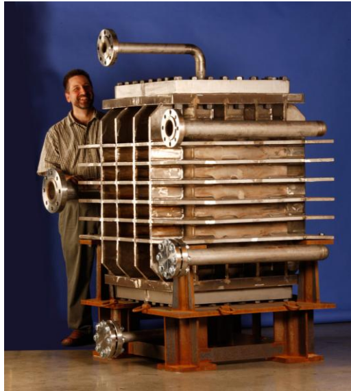
Figure 98: Reactor housing for microchannel core (Velocys, 2012b)
