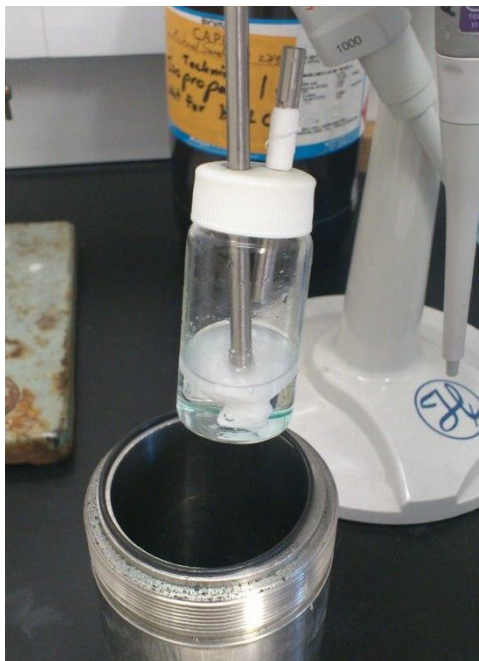
Figure 43: The glass vial inside the collection pot. The tube to the left is the inlet directly into the vial, the outlet of the vial is to the larger collection pot
