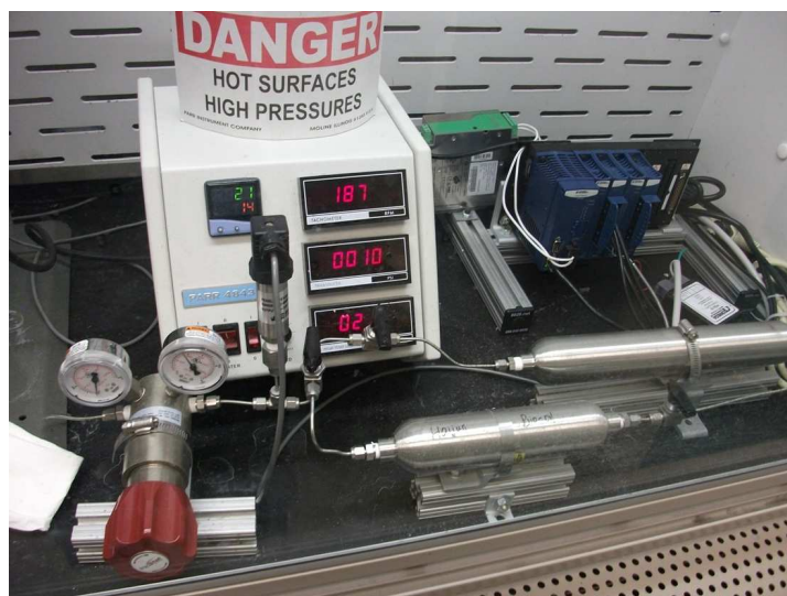
Figure 3: Reactor pressure, temperature and rpm readout/control. Note in the foreground are the syngas and the H 2 reservoirs running to the regulator
