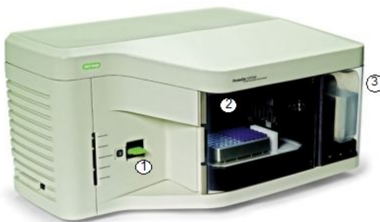
Figure 4.1: The ProteOn XPR36. 1) The chip. 2) Sample chamber containing rack and autosampler. 3) Running Buffer Chamber.
