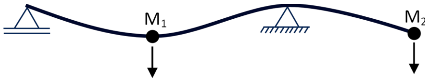
Figure 2.3 – High Energy Deflection Shape of a Beam under a Uniform Acceleration Field
