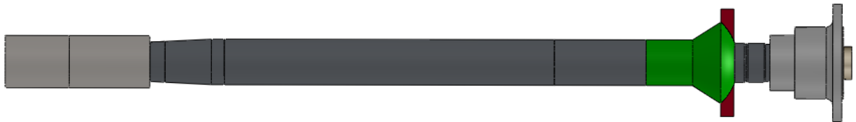
Figure 3.5 - Geometry Description of the Thrust Bearing Characterisation Model (ANSYS Workbench v14.1)
