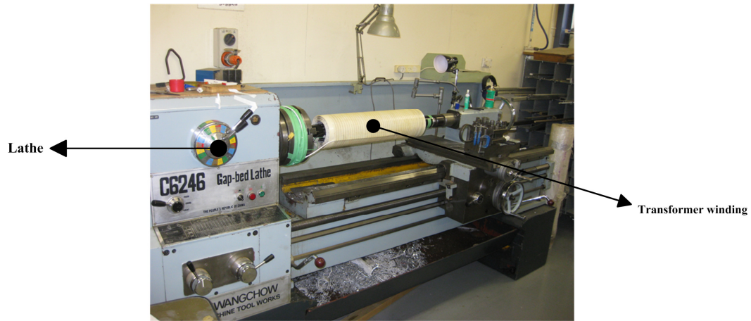
Figure 4.7 The PCPT winding construction setup.
